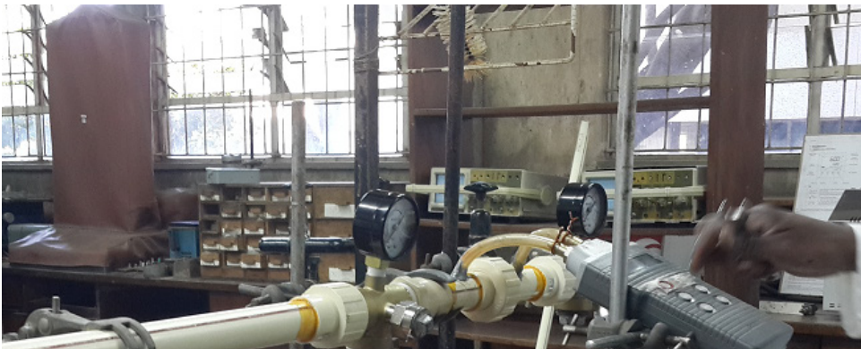
Figure 5: Shows the breathability test rig with an online Comark C9555 Dry-Use differential pressure meter calibrated to read pressure within 0-to-±210000 Pa. Upstream and down stream pressure gauges to verify pressure change before and after the cloth disc holder.
